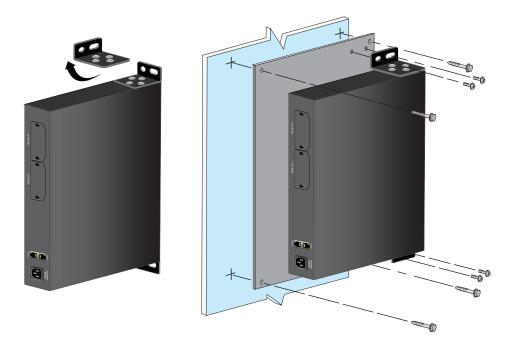
Figure 32. Wall Mounting the NetVanta 3450 and NetVanta 3458
